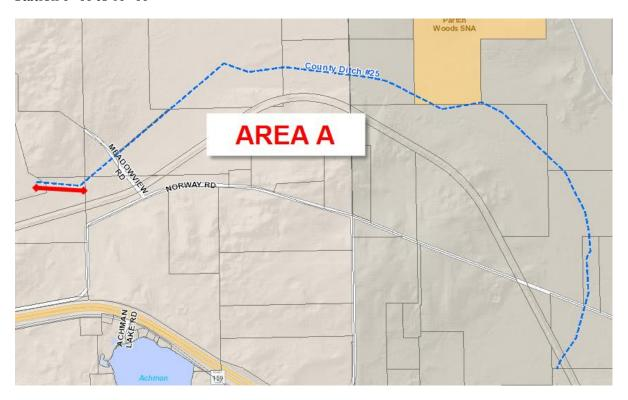
Restore entire extent of ditch to form a 4 foot bottom and 7-9 foot top of ditch width. Spot excavations are required to restore ditch to design.
