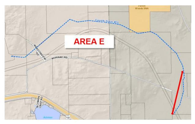
Reshape ditch to form a 4 foot bottom and 7-9 foot top of ditch width as well as spot excavations to restore ditch to design.
